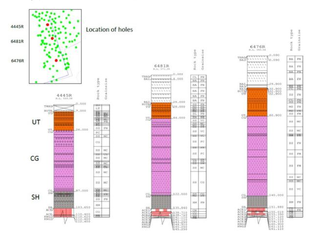
Figure 6-3: Development of simplified major material types from detailed geologic logs (for reference purposes only)
