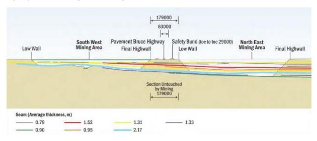
Figure 4-4: Conceptual mining section inclusive of the Bruce Highway (Cardno, 2018)
