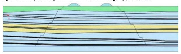
Figure 4-5: Plaxis Model section used to model high wall stability adjacent to the Bruce Highway (Cardno, 2018)
